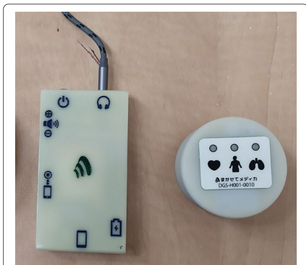
Fig. 1 The wireless stethoscope (right), allowing different auscultation modes represented by the heart and lungs icons, the receiver unit (left) with different connections available for remote transmission of auscultation data, and the speaker cable (top) that allows the physician to hear heart and lung sounds without breaking PPE protocols
